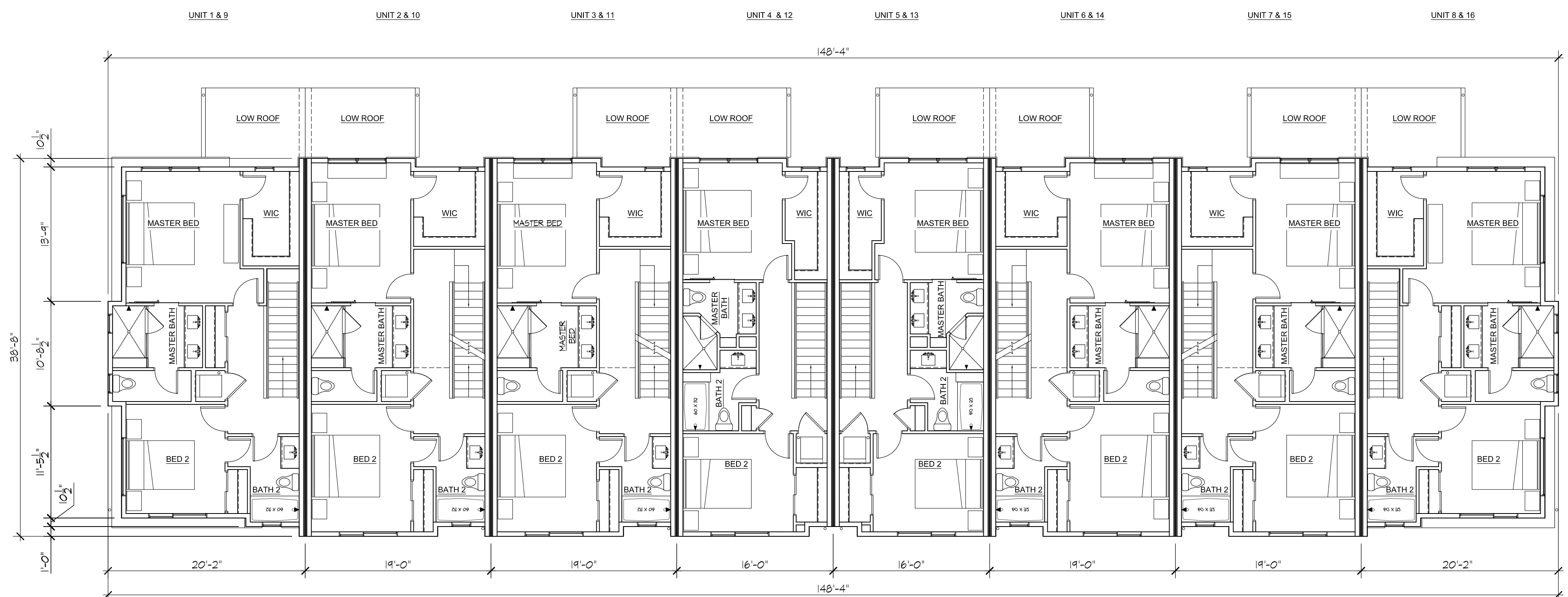
3 3RD LEVEL - BUILDING 1 & 2 SCALE: 1/8" = 1'-0"
