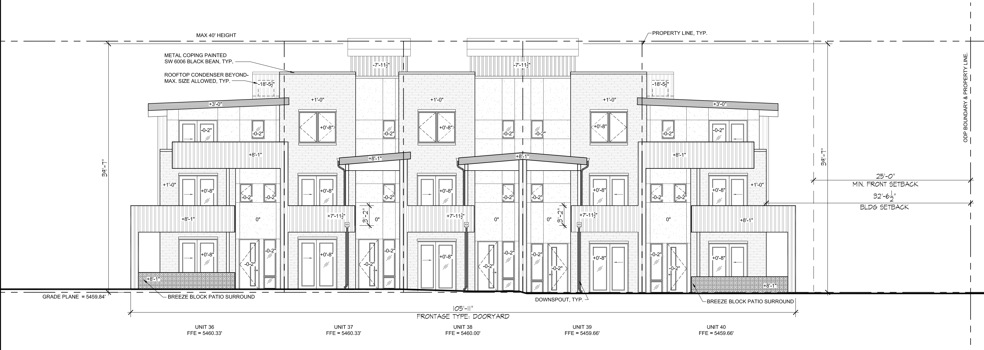
4 BUILDING 6 - EAST ELEVATION (PIERCE STREET) SCALE: 1/8" = 1'-0"
