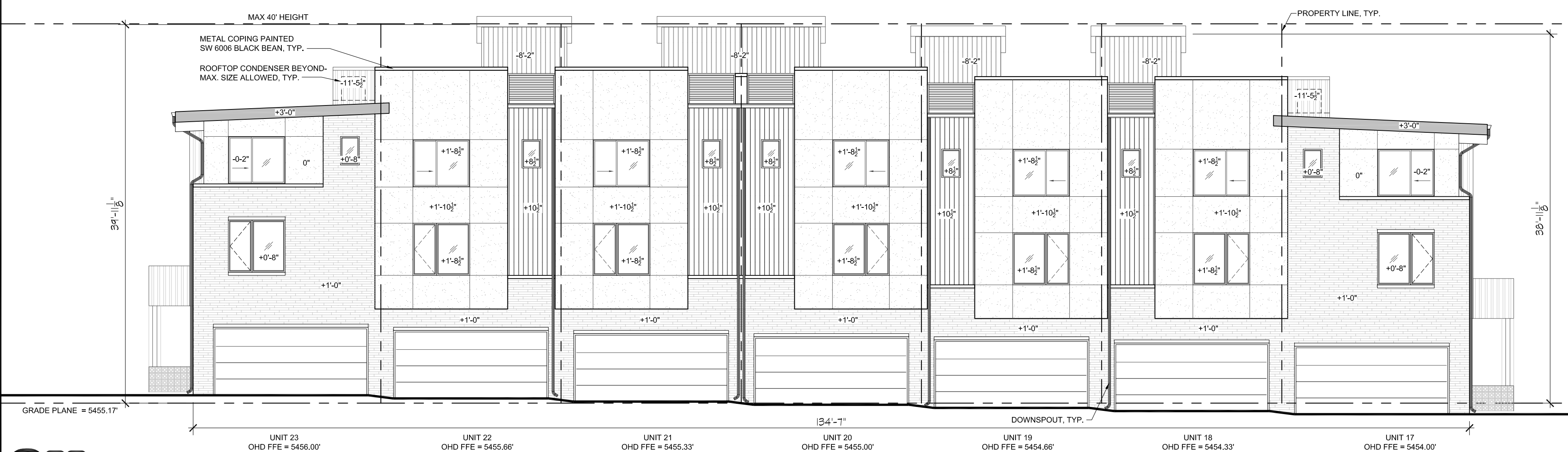
3 BUILDING 3 - NORTH ELEVATION (DRIVE AISLE) SCALE: 1/8" = 1'-0"
