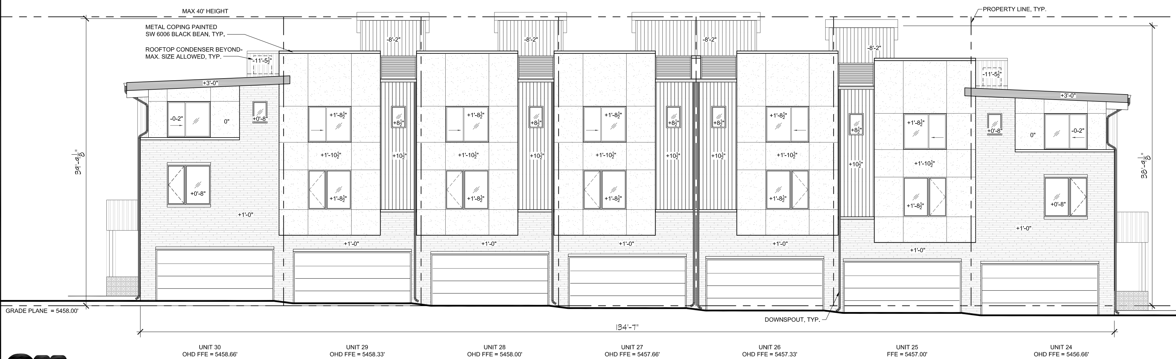
3 BUILDING 4 - NORTH ELEVATION (DRIVE AISLE) SCALE: 1/8" = 1'-0"
