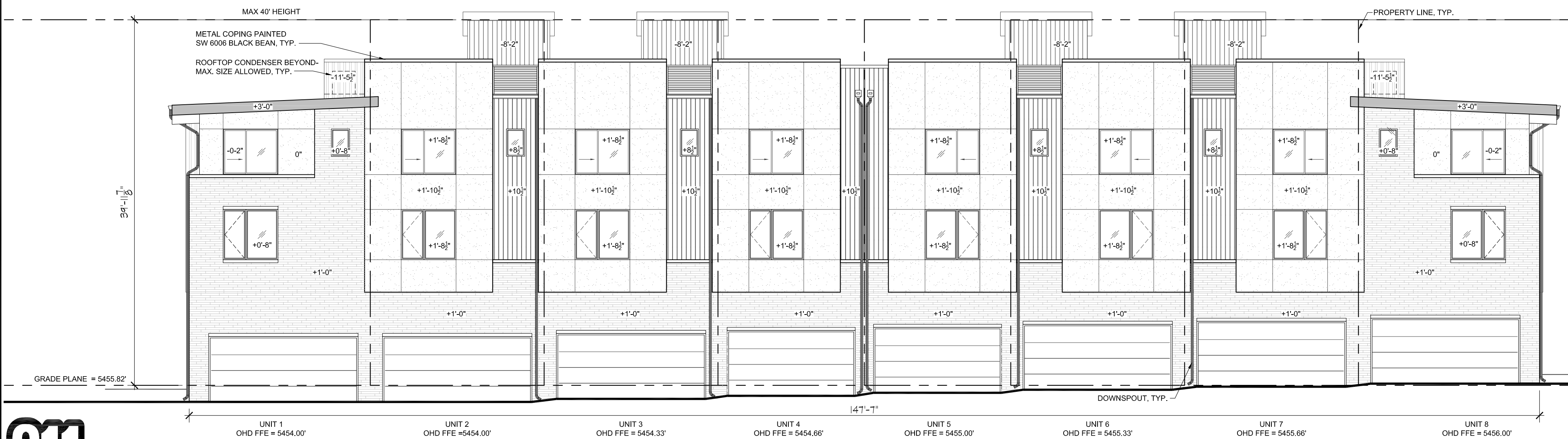
3 BUILDING 1 - SOUTH ELEVATION (DRIVE AISLE) SCALE: 1/8" = 1'-0"
