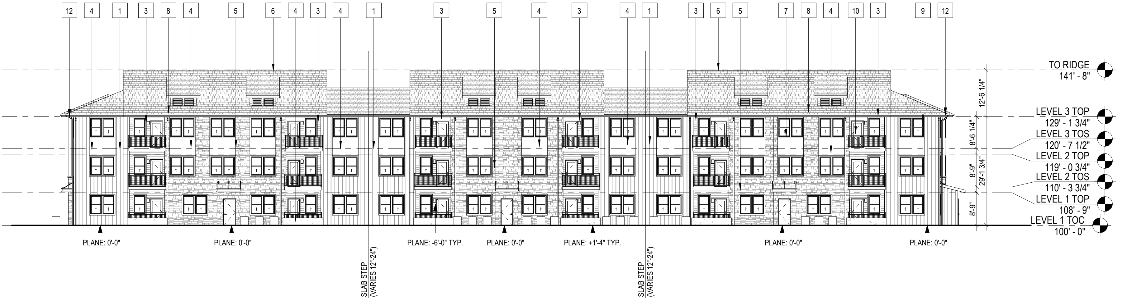
BUILDING D - ELEVATION - BACK SCALE: 1/16" = 1'-0" 1
