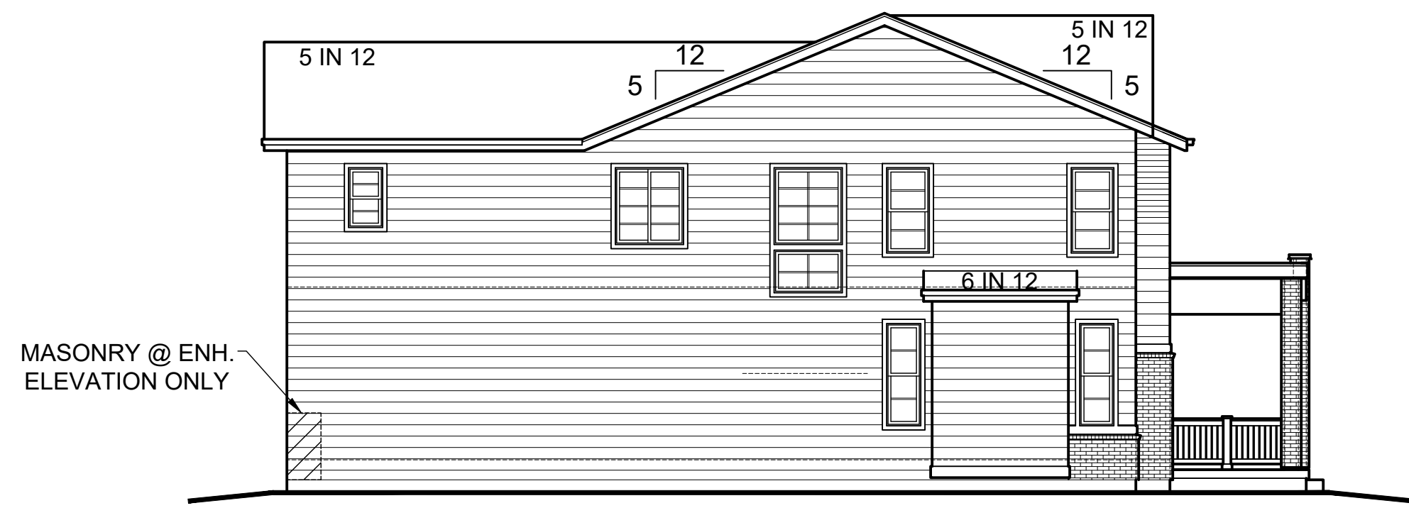
3030 ELEVATION 'D' - LEFT (PASSIVE SIDE) PASSIVE SIDE WILL NEVER BE ENHANCED SCALE: 1/8" = 1'-0"
